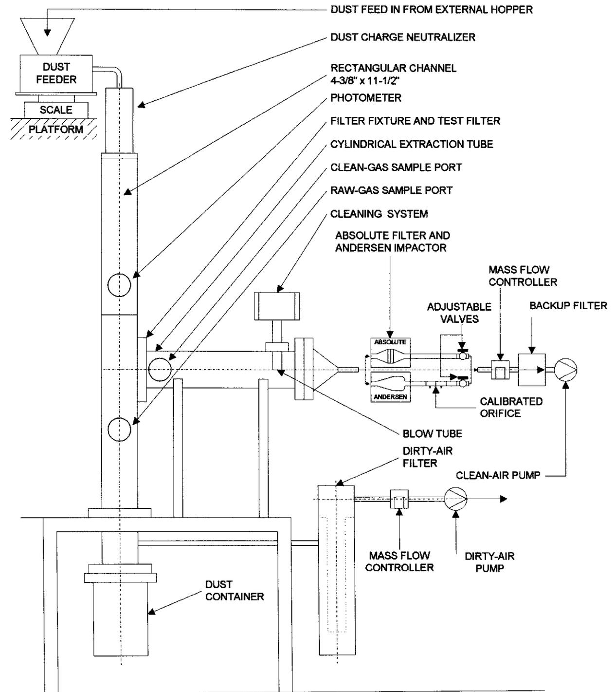
Figure 1 Filtration Performance Test Apparatus
